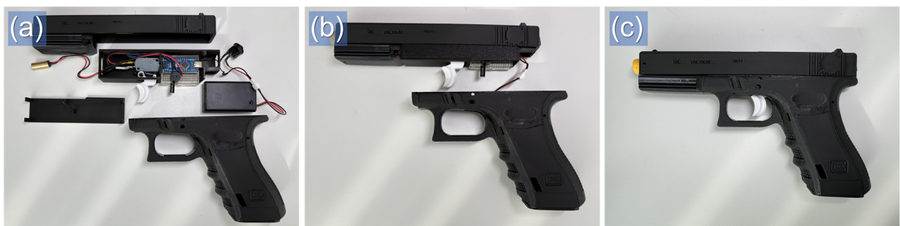
Figure 2. Laser-gun module: (a) internal view showing the circuit connections and major components; (b) partially assembled state after circuit integration into the enclosure; (c) fully assembled laser-gun module used in the experiments.
