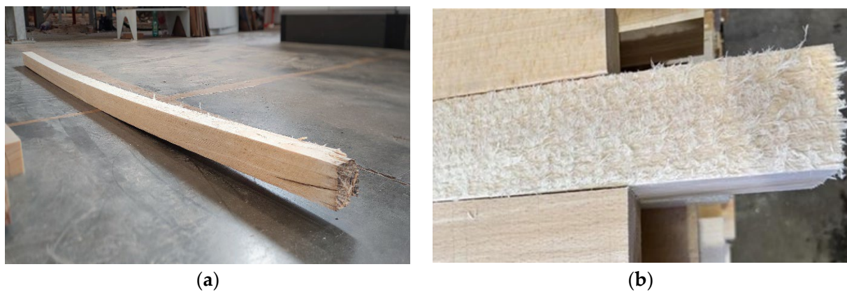
Figure 1. (a) Initial warp in the beech blanks; (b) woolly surface on specimens.
