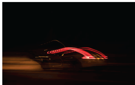
Figure 9. A demonstration of the phantom array effects in the car light [64]. Adapted from James M. Gaines, Illuminating Engineering Society (IES).
