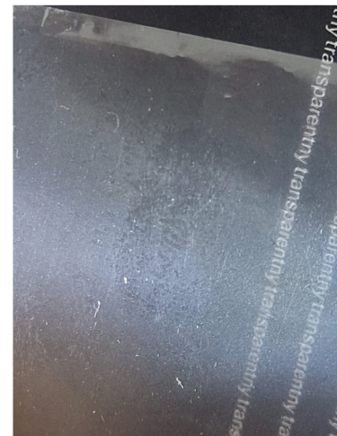
Figure 3. Oblique-light photographs of transparent silicone-coated PET release liners on a dark printed background: (a) Dolpap, (b) Crosil 42, and (c) Rossella. The printed background was intentionally retained as a qualitative contrast/scale reference and to show film transparency; images were not used for roughness or defect-density quantification.
