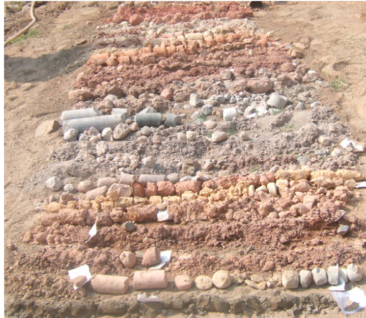
Figure 5. Selected soil–rock mixture samples in typical drilled core (drilling depth is 70 m).
