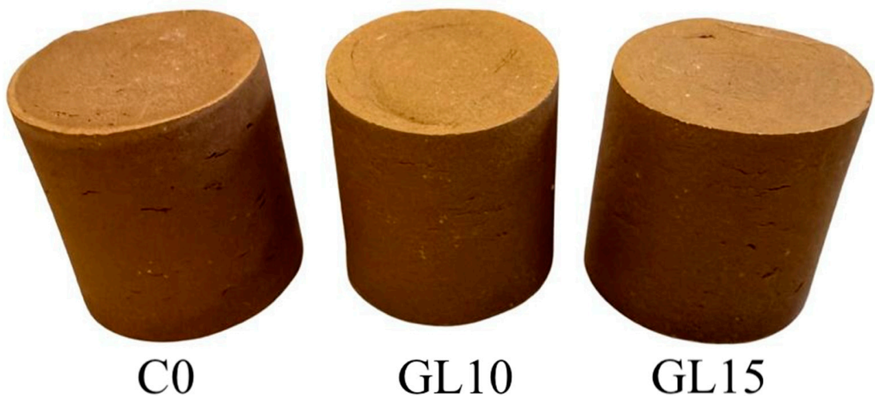
Figure 4. Appearance of the fired ceramic specimens after firing at 1125 °C, illustrating the influence of mineral additives on dimensional stability and deformation behavior.
