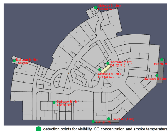
Figure 3. Fire simulation model of Dongfang Fulaide.
