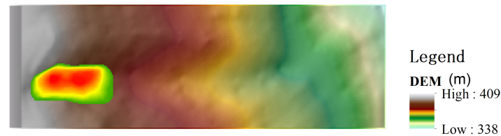
Figure 5. Initial topography and source area of the Hong Kong landslide case adopted in this study.
