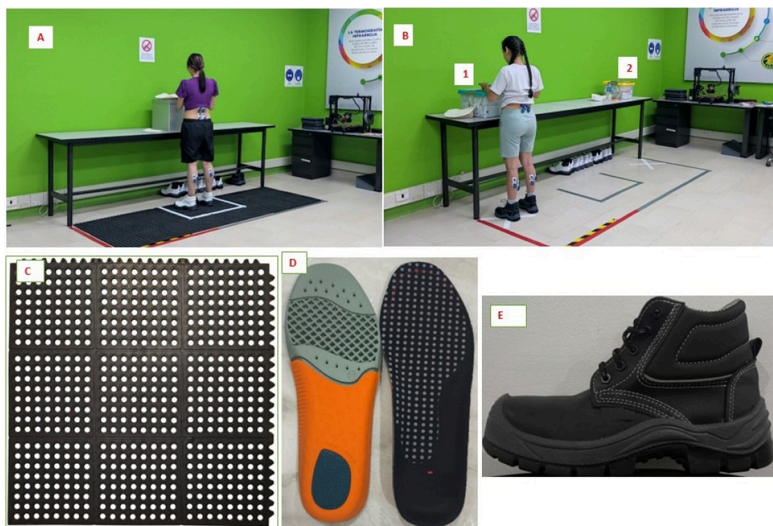
Figure 2. Experimental factors. (A): Static posture. (B): dynamic posture. (C): anti-fatigue mat. (D): insole inserts. (E): safety boots.
