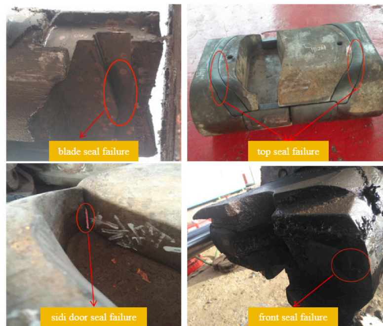
Figure 2. Ram seal failure location.
