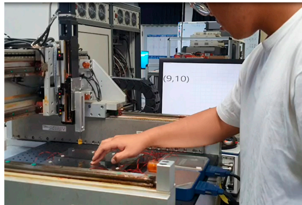
Figure 10. A photo showing field test on the tactile sensing glass plate by a volunteer.
