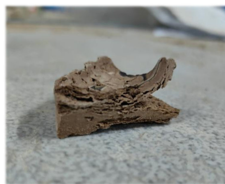
Figure 15. Dried soil sample near the anode in the group with 1% slag and 0.6% APAM.
