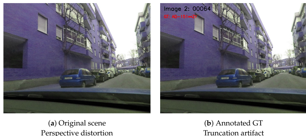
Figure 7. UC3M-LP Test Image 2. (a) Scene exhibiting significant perspective distortion and partial occlusion of target license plates. (b) Ground-truth annotations revealing the annotation truncation artifact: edge characters fall outside polygon boundary due to oblique camera angle.
