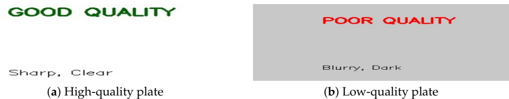
Figure 14. Image quality impact on recognition accuracy. (a) High-quality plate ( Q(I) > 200 , contrast > 0.6 ) achieves A4 accuracy \geq 95\% . (b) Low-quality plate ( Q(I) < 80 , contrast < 0.3 , motion blur) achieves A4 accuracy 65–75%.
