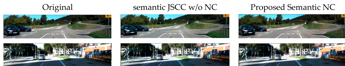
Figure 4. Representative visual reconstruction results on the KITTI high-resolution test set under the AWGN channel at 7 dB. The first column shows the original KITTI test images, while the remaining columns compare the reconstructed images obtained by semantic transmission without NC and the proposed semantic NC scheme, respectively.
