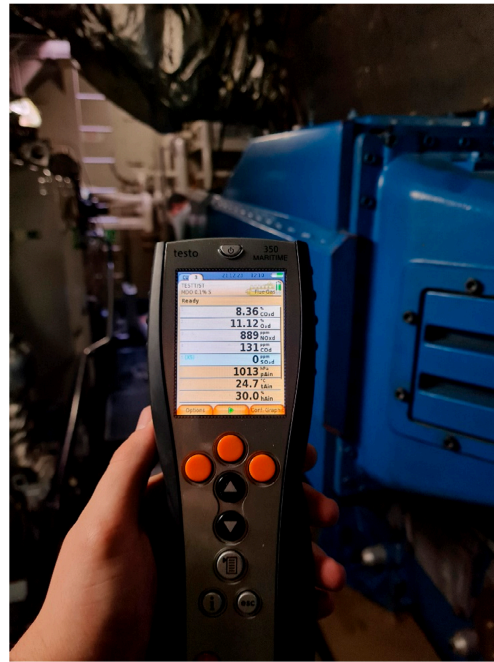
Figure 6. Real-time display on the Testo 350 MARITIME handheld control unit during reading of NO x and other pollutants in exhaust emissions.
