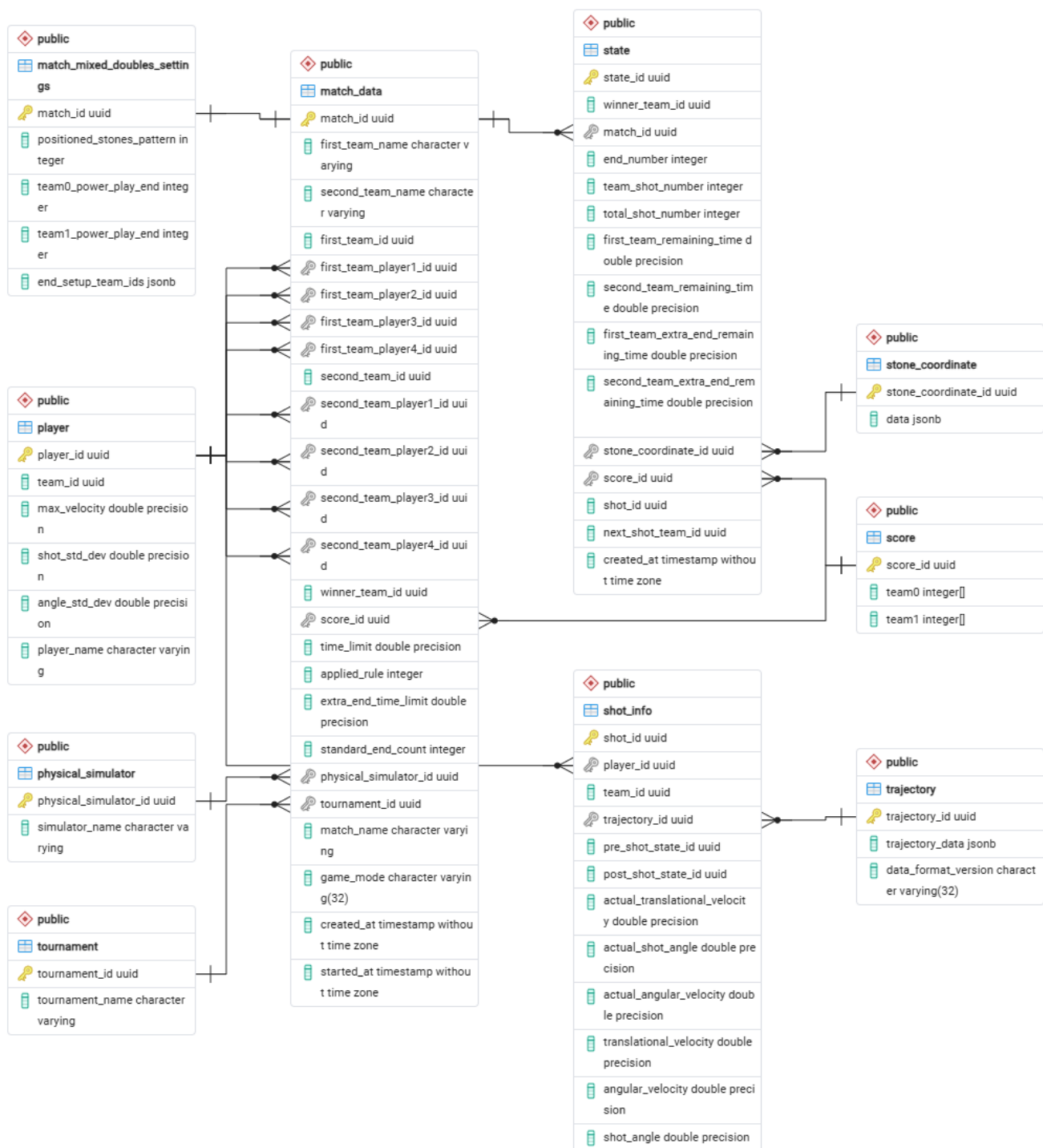
Figure 4. Entity–relationship diagram of the database schema. Match metadata, per-shot states, shot history, and recorded trajectories are linked by foreign keys, and mixed-doubles-specific configuration is isolated in the match_mixed_doubles_settings table.
