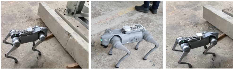
Figure 14. Activation and operation of the Unitree Go2 quadrupedal robot during experimental inspection tests.
