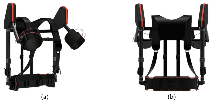
Figure 1. Physical schematic of the upper-limb exoskeleton: (a) Front view of the exoskeleton; (b) Back view of the exoskeleton. The device weighs 1.9 kg and uses a passive spring-based elastic energy storage mechanism to provide assistive torque during shoulder elevation. The maximum assistive torque is 15 N·m.
