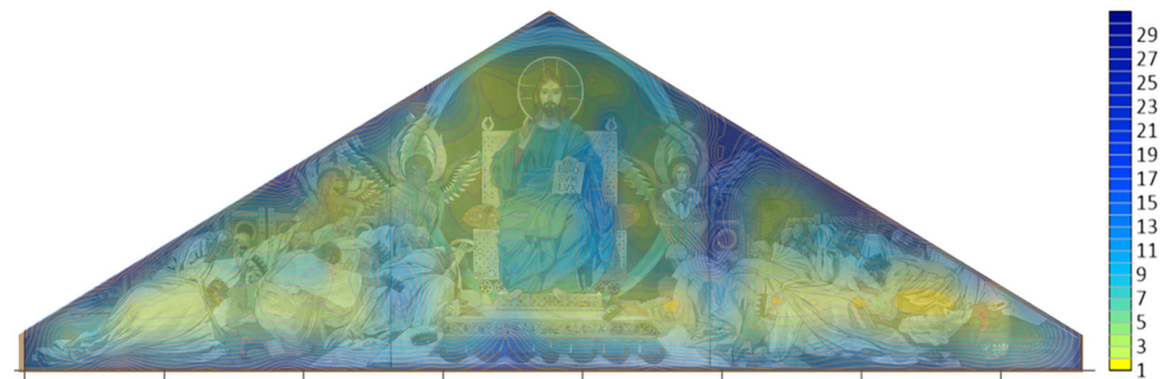
Figure 3. Hygrometric tomography generated for Cristo in Trono painting. The color scale on the right shows the moisture content detected with the instrument placed in contact with the canvas surface.
