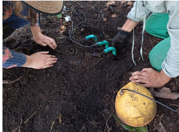
Figure 1. Installation of the 7-in-1 sensor array and the CropX multi-depth probe within the same soil pit.
