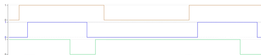
Figure 3. Test 1—cyclic toggling sequence of three output bits.
