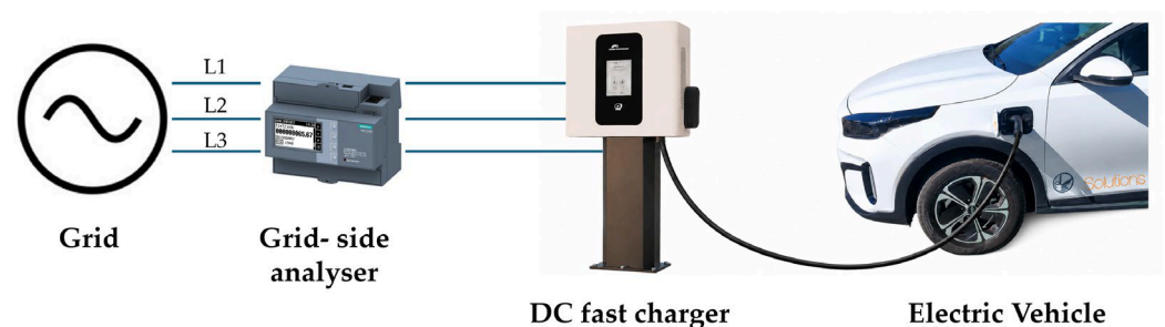
Figure 1. Schematic representation of the DC fast-charging installation and measurement points (grid-side analyser and charger side) used in the dataset. L1–L3 denote the three phases of the three-phase electrical connection.
