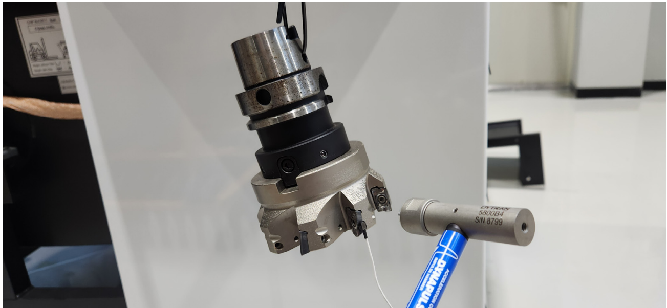
Figure 12. Natural frequency measurement.
