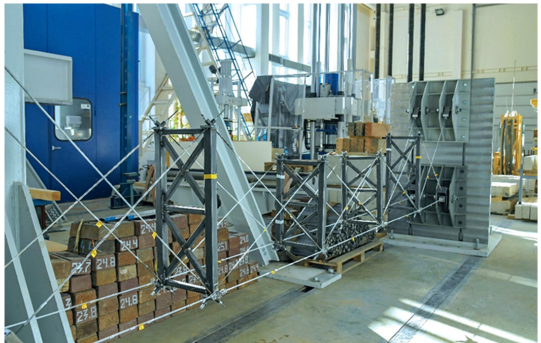
Figure 9. Cable-stayed bridge model.
