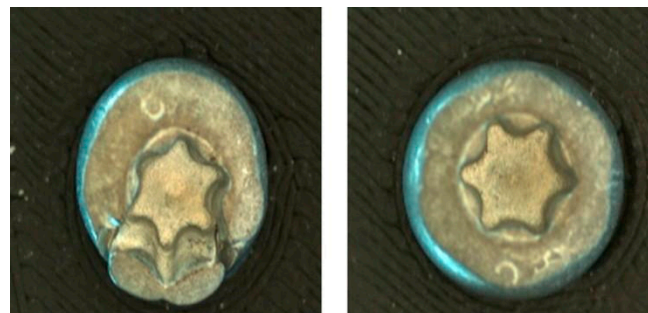
Figure 4. Examples of Defective and Non-Defective Bolts.
