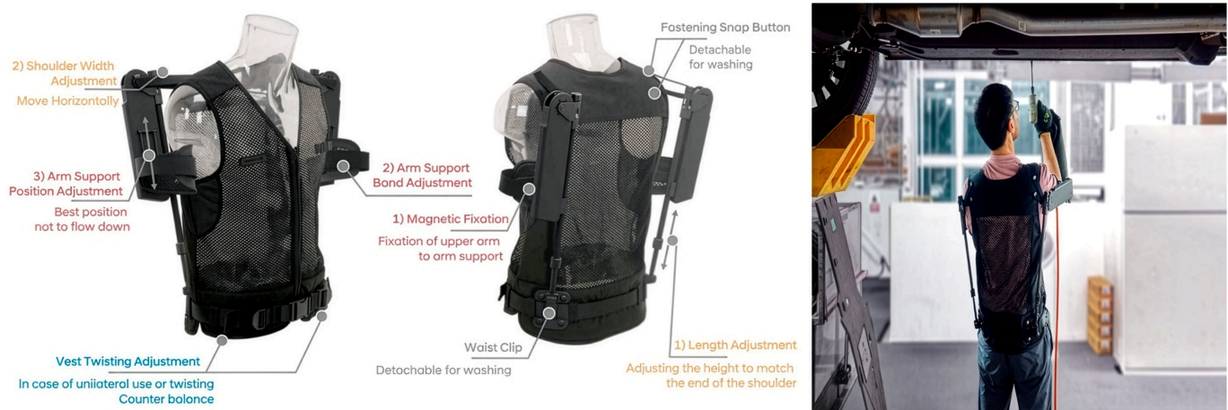
Figure 1. Structure of X-ble shoulder and appearance while wearing.
