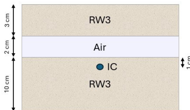
Figure 1. Schematic representation of the heterogeneous phantom employed for the validation.
