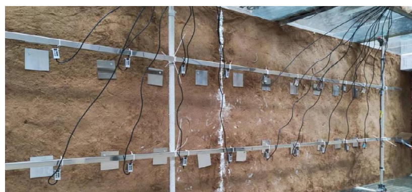
Figure 3. Field layout photo of displacement meters.
