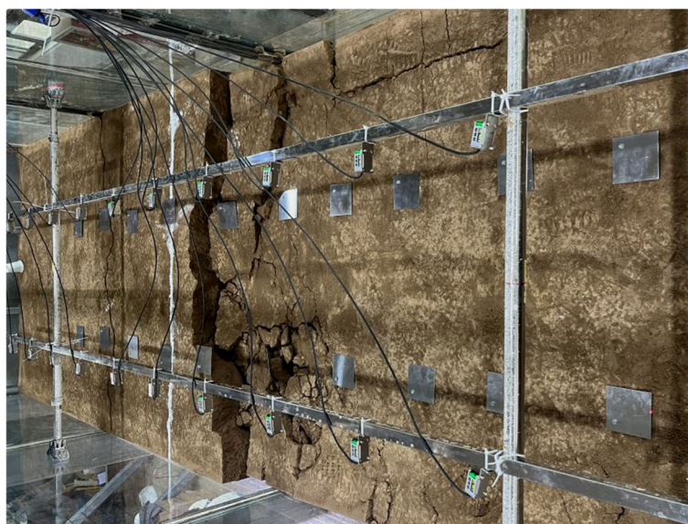
Figure 6. Live photograph of surface rupture propagation (taking Case 4 as an example).
