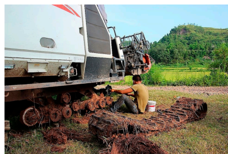
Figure 9. Track disassembly for field repair (illustrative photograph).
