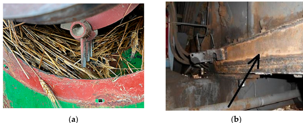
Figure 6. (a) Severe blockage of the threshing drum [64], (b) Crack on the left side of the thresher frame (in the direction of the arrow, a reinforcing plate applied) [5].
