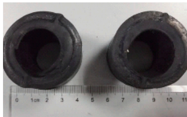
Figure 7. Rubber bearing wear diagram [65].
