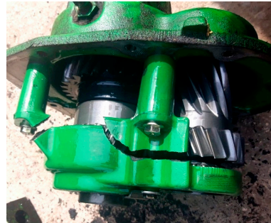
Figure 8. Break in the gearbox cover [5].
