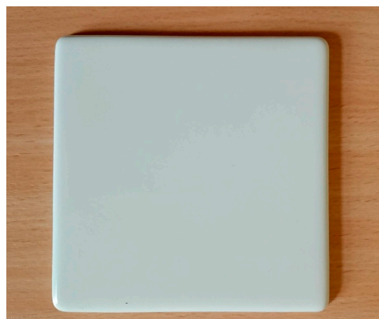
Figure 3. White enamel standard no. LX17112 by HunterLab.
