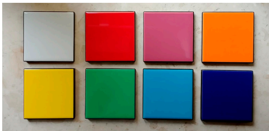
Figure 1. Set of ceramic color standards (DM05) used during the experiment (pale gray, red, deep pink, orange, yellow, green, cyan, and deep blue).
