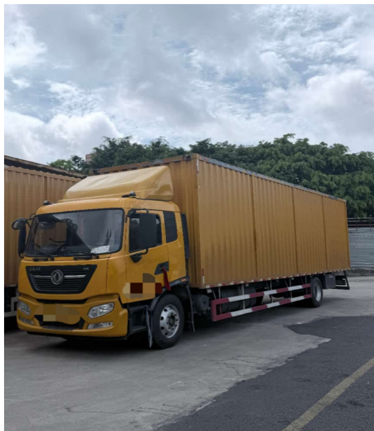
Figure 6. The 2025-model Dongfeng Tianjin KR Plus 4 \times 2 box truck (DFH5170XXYEX16), manufactured in 2026, powered by a Dongfeng DDi75E300-60 diesel engine, and used in the roadside acoustic experiment.
