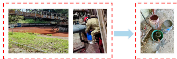
Figure 1. Tailings Sampling Procedure at the Mineral Processing Plant of Daye Iron Mine.
