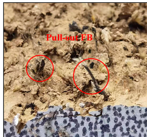
Figure 12. Fiber pull-out morphology on fracture surfaces.
