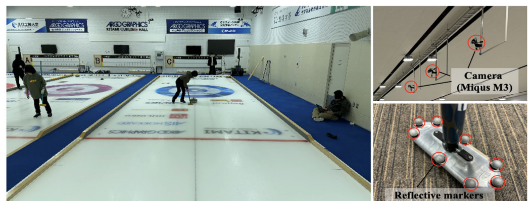
Figure 5. Scene of the experiment (left). Motion capture camera and reflective marker settings (right).
