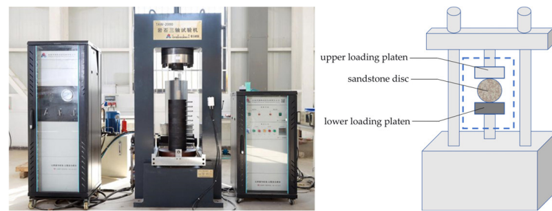
Figure 1. Brazilian splitting test apparatus and schematic diagram.
