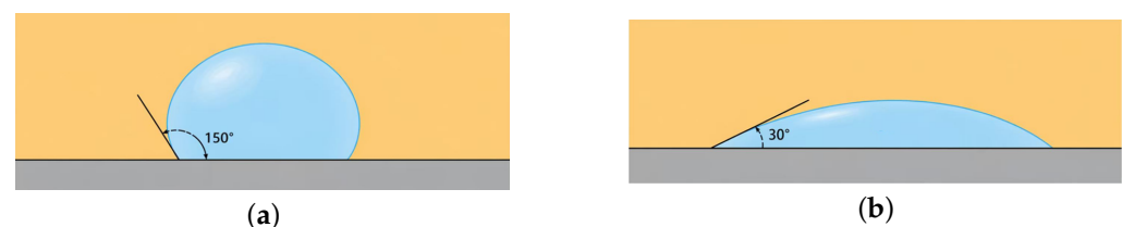
Figure 3. Definition of the primary-phase contact angle used in the simulations: (a) large primary-phase contact angle; (b) small primary-phase contact angle. The blue region denotes the primary phase, the yellow region denotes the secondary phase, and the contact angle is measured through the primary phase.
