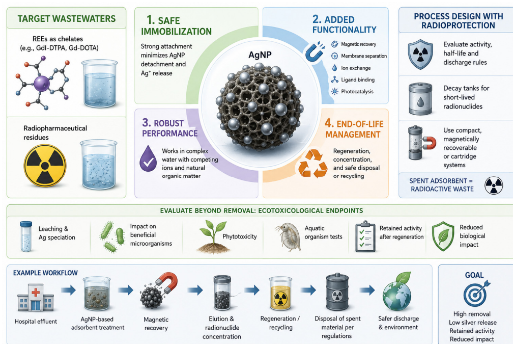
Figure 4. Conceptual framework for the safe-by-design development of silver nanoparticle (AgNP)-based platforms for the treatment of rare earth element (REE)-containing wastewater and radiopharmaceutical residues. The scheme highlights the four key design principles: (i) stable immobilization of AgNPs to minimize silver release; (ii) integration of support-specific functionalities (e.g., magnetic recovery, membrane separation, ion exchange, ligand-assisted binding, or photocatalysis); (iii) robust performance under complex wastewater conditions; (iv) end-of-life management through regeneration, selective concentration of contaminants, and safe disposal or recycling. The workflow also emphasizes the importance of evaluating ecotoxicological endpoints, including silver leaching, biological impact, regeneration efficiency, and environmental safety, alongside contaminant removal performance.
