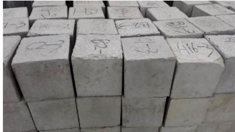
Figure 1. Standard specimens used for moisture absorption and desorption tests.
