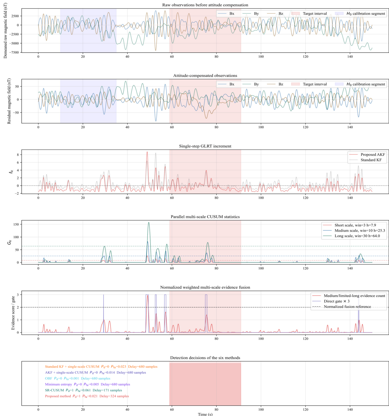
Figure 2. Example of a typical single-run detection process at \text{SNR} \approx 2.7 with six detection methods.
