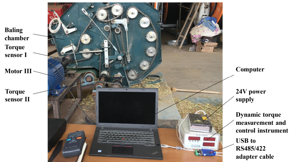
Figure 5. Bale chamber test system assembly.
