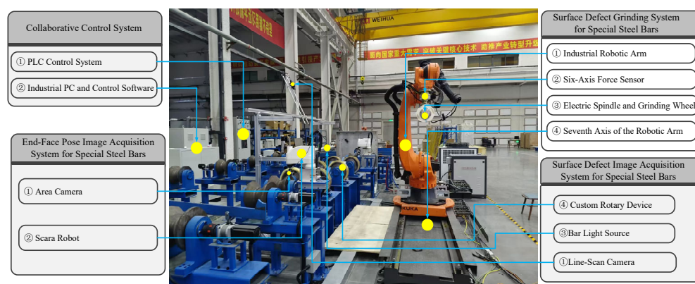
Figure 1. Schematic of the surface defect image acquisition and robotic grinding system for special steel bars.
