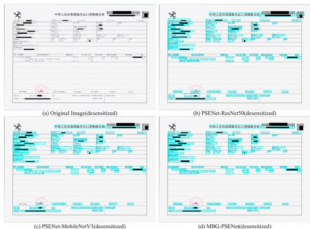
Figure 8. Comparison of detection results among different models. Sensitive information in the customs declaration image has been masked with black rectangles for privacy protection, and the cyan boxes indicate the text regions predicted by each model.
