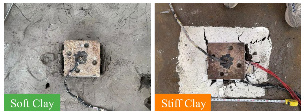
Figure 19. Ground surface deformation after shaking table test.
