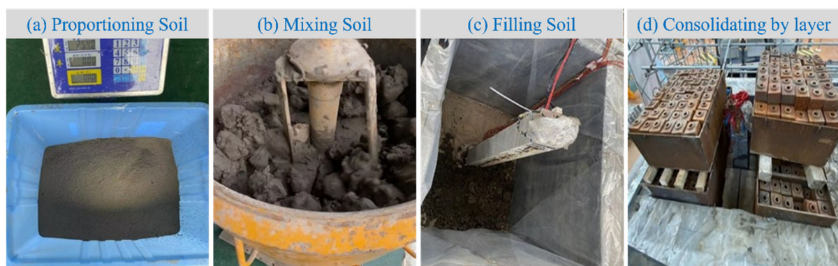
Figure 7. Model soil preparation and layered filling.
