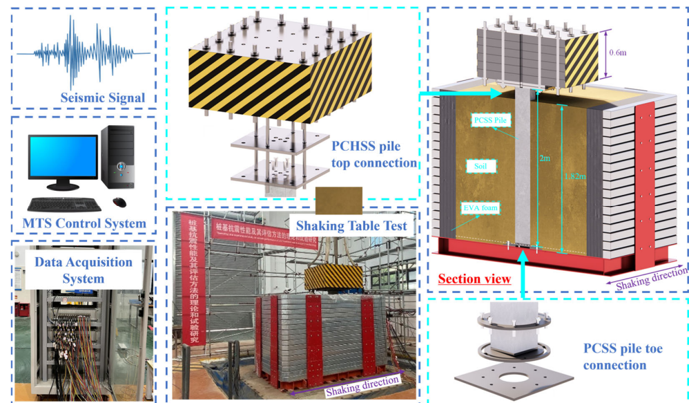
Figure 1. Shaking table test setup.
