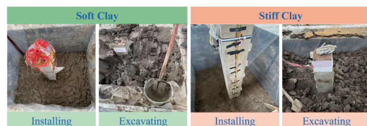
Figure 8. Soil photos in the laminar box.
