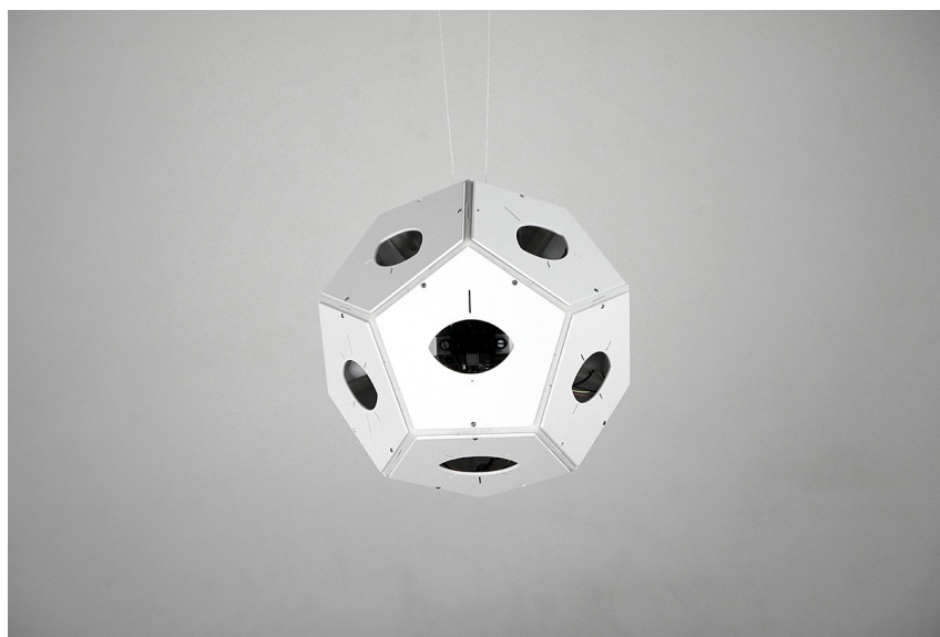
Figure 2. The Dodecaudion—a perfect “blank canvas” for experimentation on various sensor-to-sound mappings.
