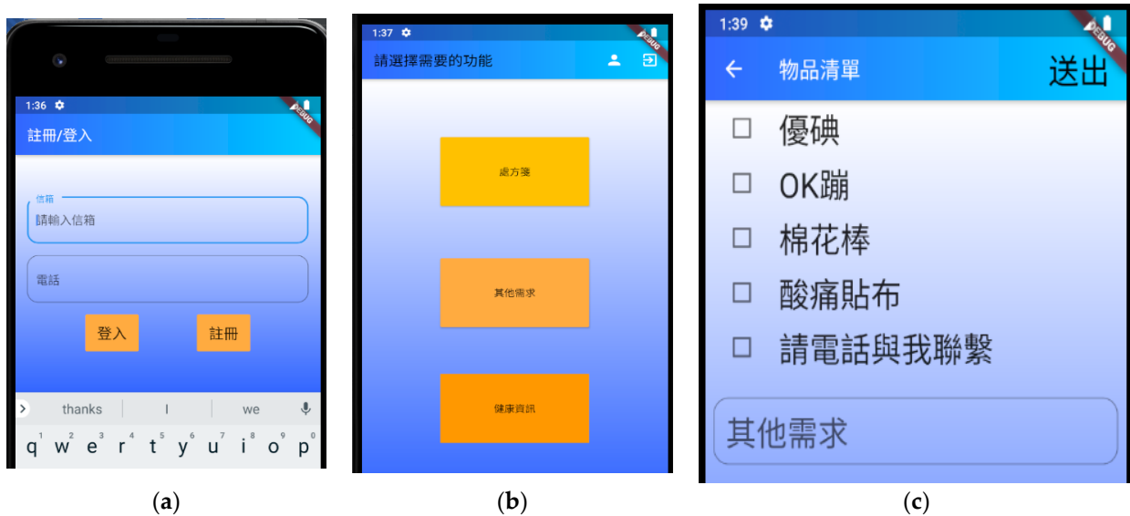
Figure 3. Main interface and functions design in traditional Chinese character. (a) is registration and login in screen by key in phone number; (b) is function selection, three large buttons provide medicine, daily necessities, and health consultation respectively; (c) provide items selection without input words.
