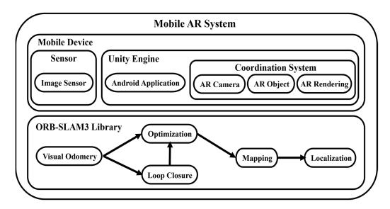
Figure 4. Proposed Mobile AR System Structure.
