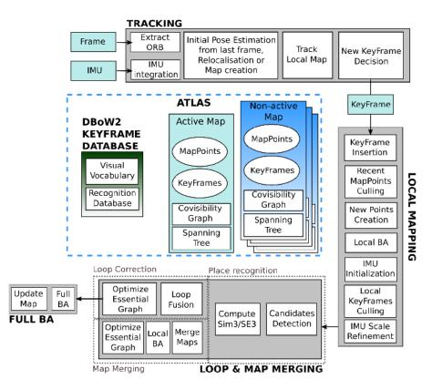
Figure 3. ORB-SLAM3 System Structure.
