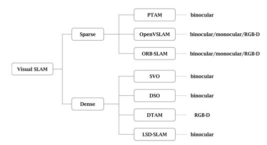
Figure 2. Classification of the Visual SLAM Technologies.
