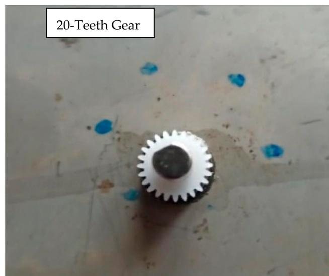
**Figure 21.** Teeth gear to slow down the RPM.
