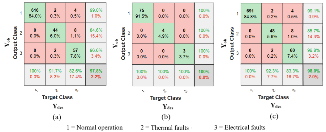
Figure 11. Confusion matrix for classifying the three classes (1—normal operating condition, 2—thermal faults, 3—electrical faults) obtained by PRN with 10 neurons in the hidden layer, (a) training phase with 90% of samples (733), (b) validation phase with 10% of samples (82), (c) 100% of samples (815).
