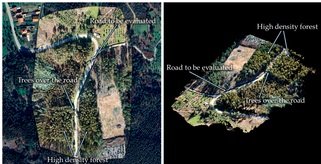
Figure 7. Orthophoto and 3D point cloud of the Castanheira use case.
