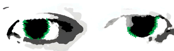
Figure 6. Results of iris edge point extraction, demonstrating the successful detection of iris boundaries for subsequent pupil center localization.
