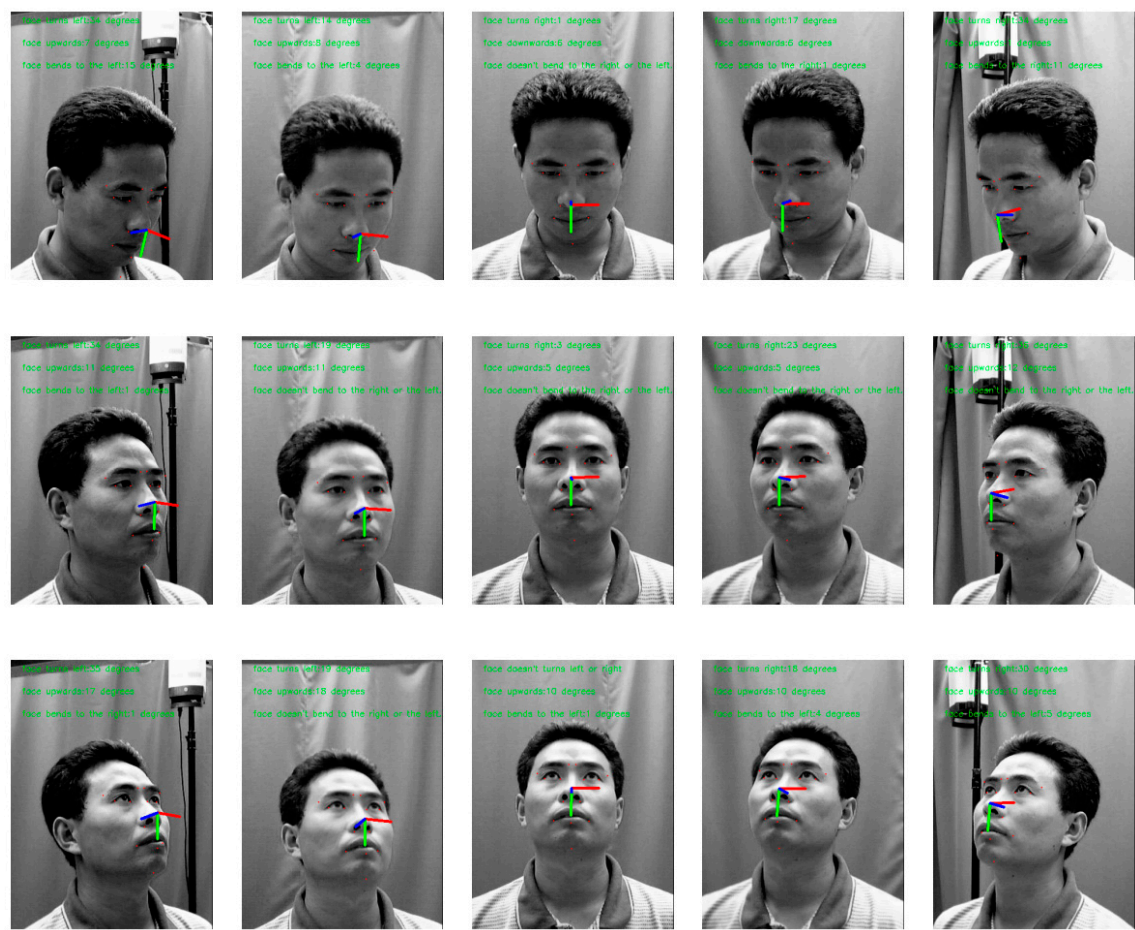
Figure 18. Head pose estimation results visualized on test images, demonstrating the estimated 3D head orientation vectors overlaid on the detected facial regions.
